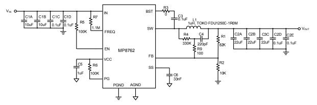
Figure 53 — Typical Application Circuit with Low ESR Ceramic Capacitor V<sub>IN</sub>=12V, V<sub>OUT</sub>=5 V, I<sub>OUT</sub>=10A, F<sub>SW</sub>=800kHz
