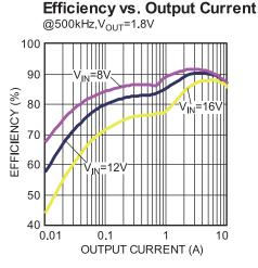
Figure 40 — Efficiency Curve
