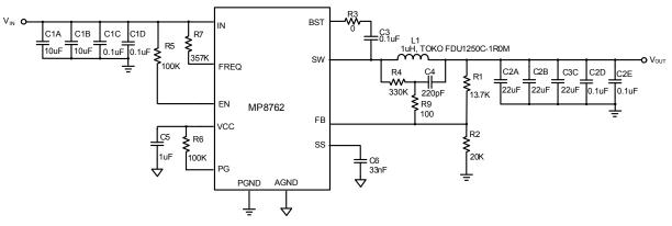
Figure 14 — Typical Application Circuit with Low ESR Ceramic Capacitor
