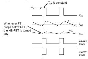
Figure 2—Heavy Load Operation
