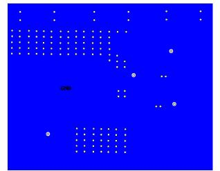
Bottom Layer Figure 57—PCB Layout Guide for MP8761GLE (16-Pin QFN)
